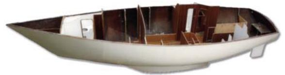
*Caliber Multi-Bulkhead Bonding System™*
