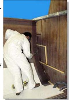
Our Multi-Bulkhead Bonding System™ is a painstaking construction method but it adds greatly to a Caliber's durability and seaworthiness. A Caliber is able to carry the load of stores for offshore voyaging, and the loads of the sea.
