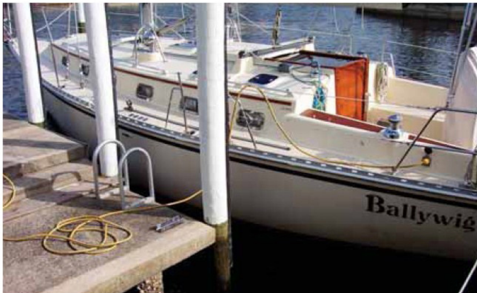
Ballywig at the dock, showing many of its features, including inboard genoa tracks and ample opening ports and hatches.
